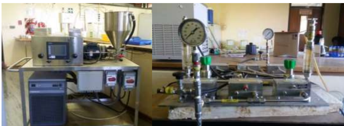
Figure 4: Crossflow assessment equipment (four and six cell set-ups) for flatsheet membranes with temperature controls
