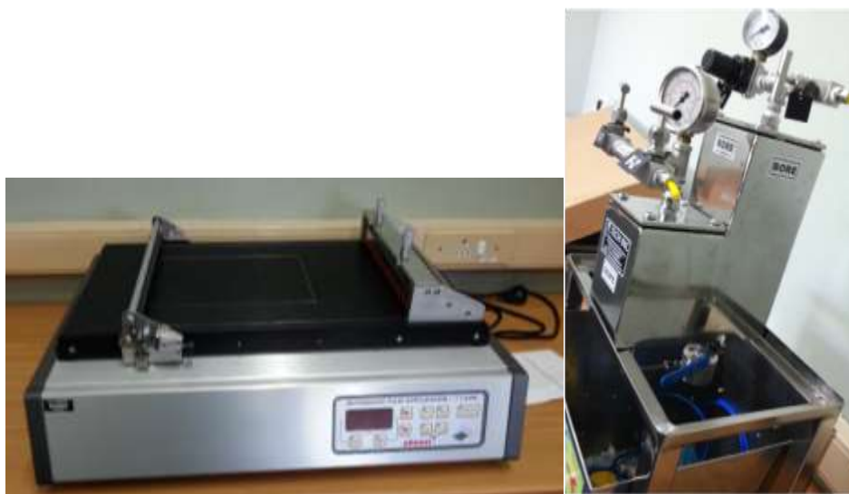
Figure 2: Automated flatsheet membrane casting equipment and a capillary membrane forming unit
