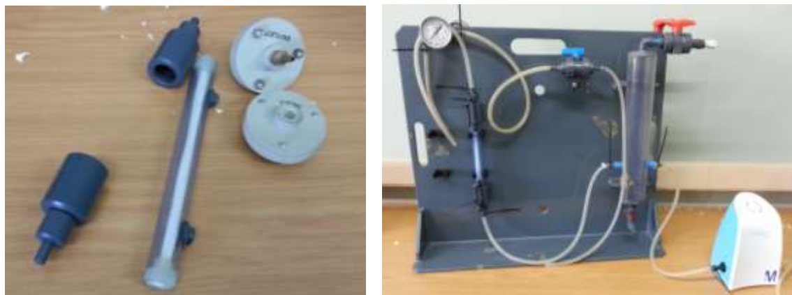
Figure 5: Flatsheet and capillary membrane modules and a benchtop assessment unit for both module types
