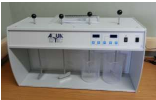
Figure 1: Jar test to assess commercial polymers for pre- and post-treatment protocol development
