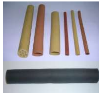
Tubular ceramic membrane prepared locally from natural materials (carbon, clay, apatite, zeolite, sand)
