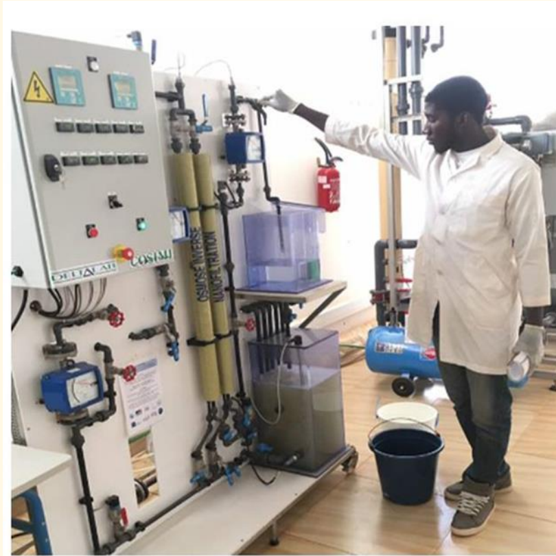
PhD candidate performs testing on NF/RO pilot equipment
