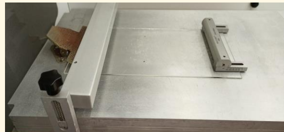
Drying by integrated suction system to evaporate the solvent
